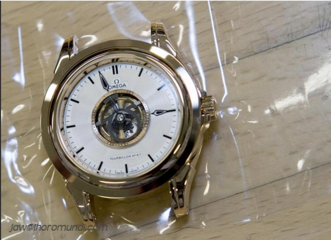
Pull the crown with a slight rotation. Once the crown is pulled out the hands can be adjusted
